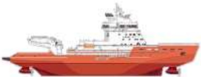
ARC 130-type LNG-fueled icebreaker (21 MW, 40 MW, 60 MW)
